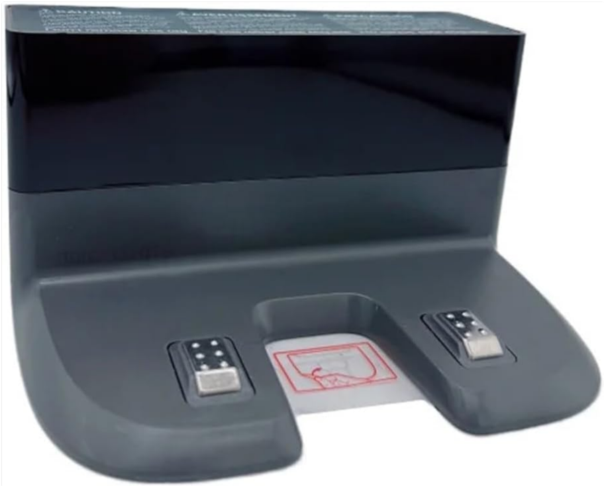
Figure 5.1: Close-up of the charging contacts on the dock. These contacts must align with the robot's contacts for successful charging.
