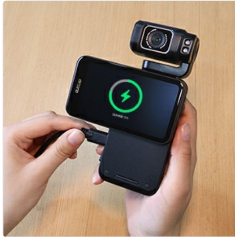
Figure 2: Charging the ORDRO M3 camcorder using the USB Type-C port.
