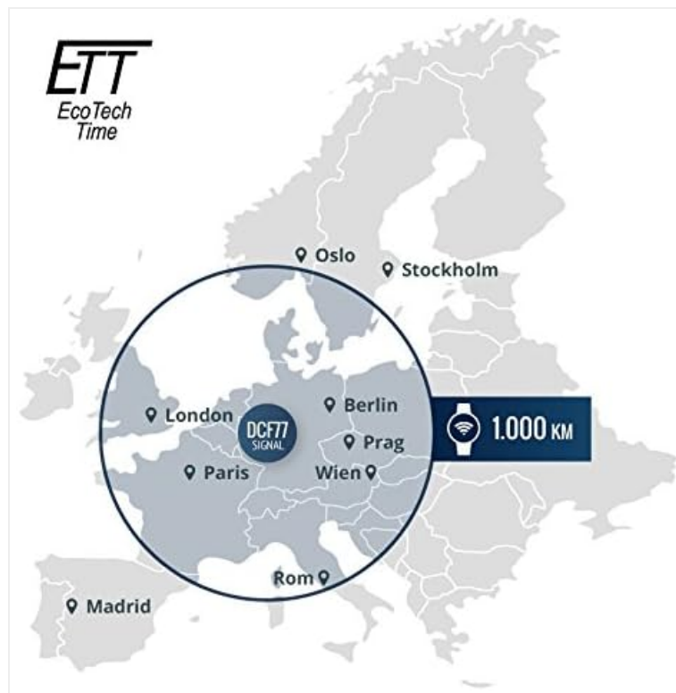
Figure 2: Approximate reception range for the DCF 77 radio signal, covering much of Europe.
