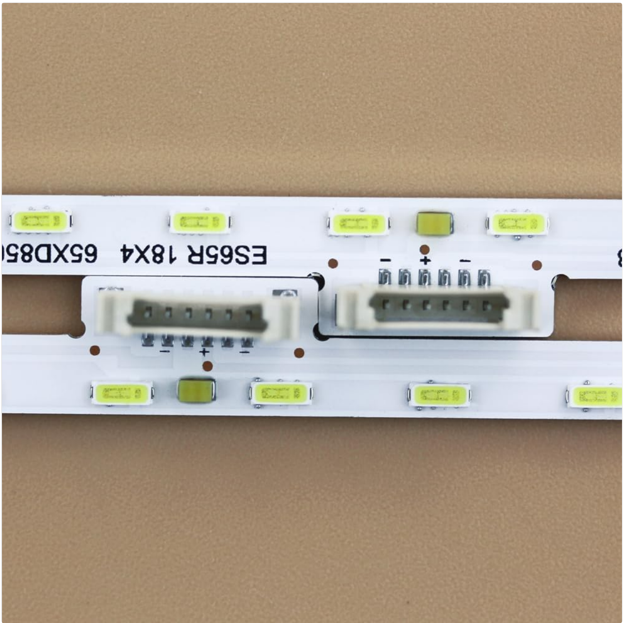
Figure 3.3: Detail of the electrical connectors on the LED backlight strip.
