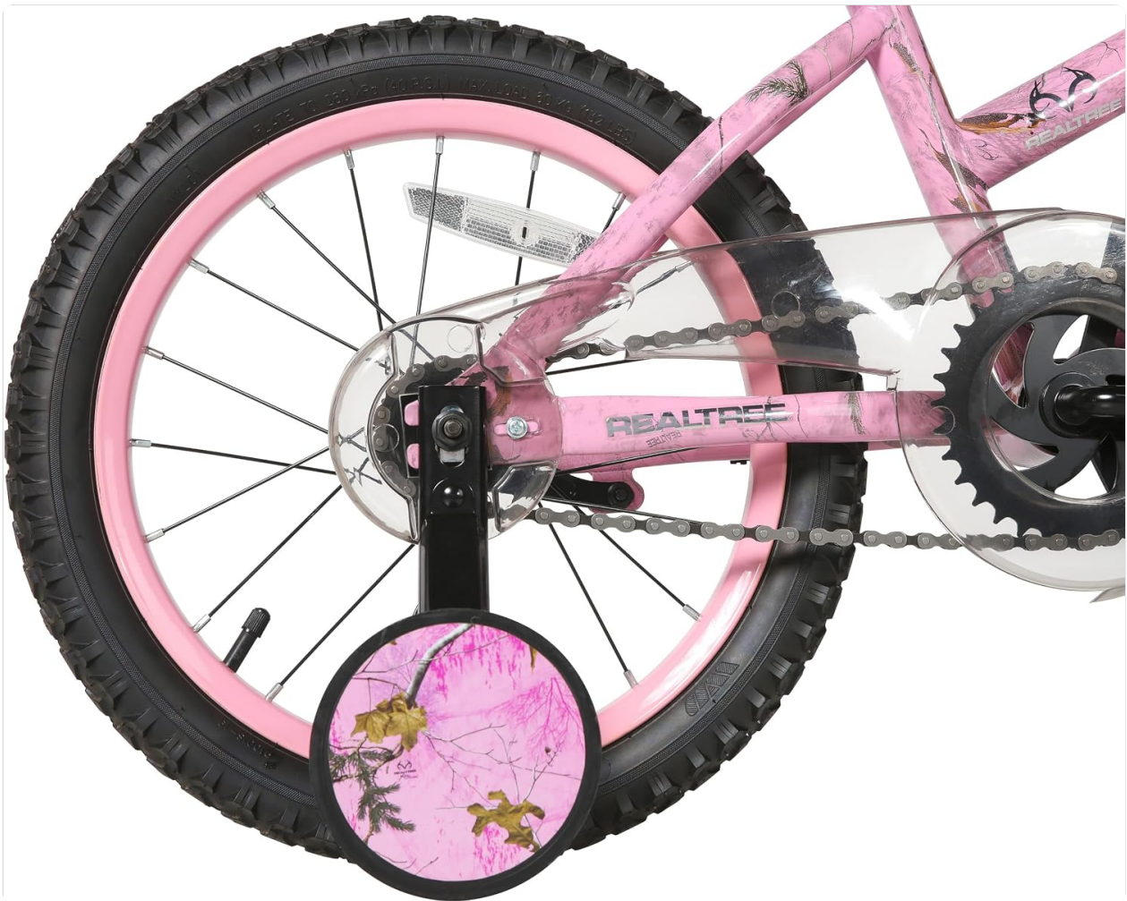
Image: A detailed view of the bike's rear wheel, showing the chain, sprocket, and the attachment mechanism for the training wheel.
