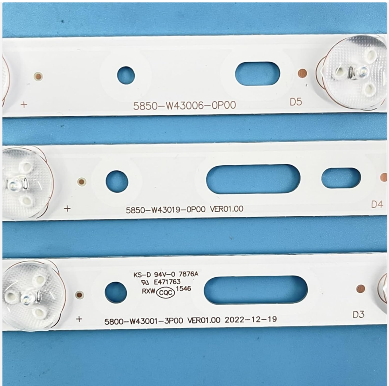
Image: A close-up showing the individual LED lenses and circuit board markings, including part numbers like 5800-W43001-3P00.
