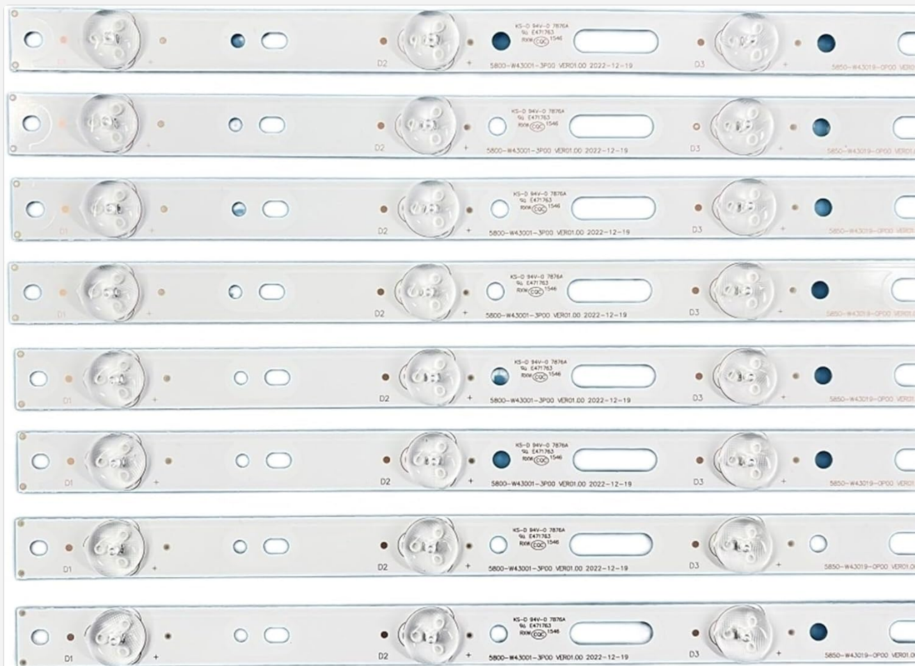
Image: A set of LOTOAK LED backlight bar strips, showing their uniform design and individual LED placement.
