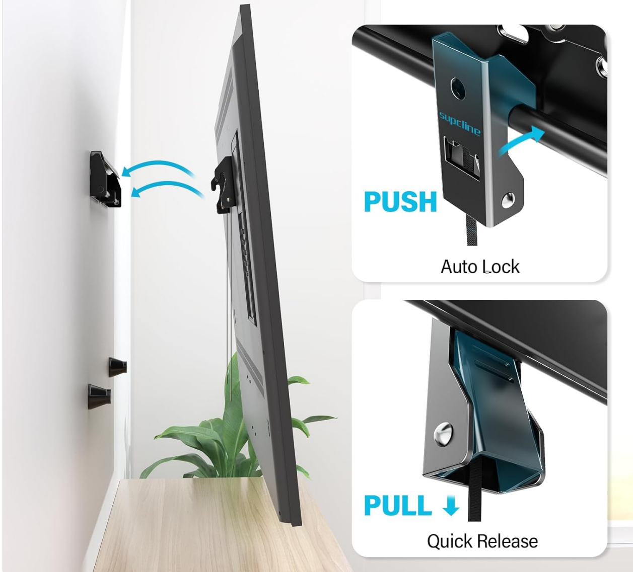
Figure 6: Auto Push Lock & Quick Pull Release. This diagram illustrates the 'Straightforward Setup' and operation of the mount's locking mechanism. It shows how to 'PUSH' the TV into place for auto-lock and 'PULL' the straps for quick release, simplifying the process of attaching and detaching the TV.
