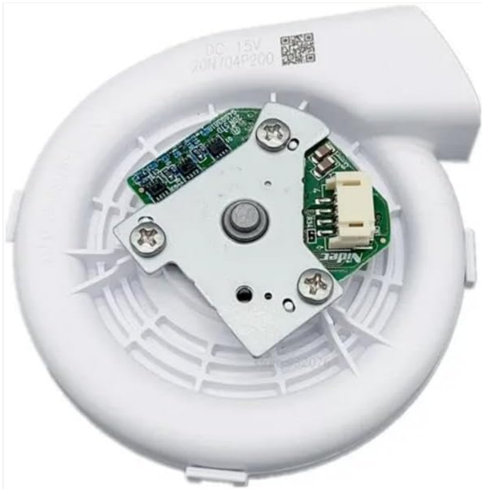
Image 2.4: Top-down view of the electric fan's internal components. This view provides a clearer look at the motor, circuit board, and the fan's internal structure, including the DC 15V and 20N704P200 markings.
