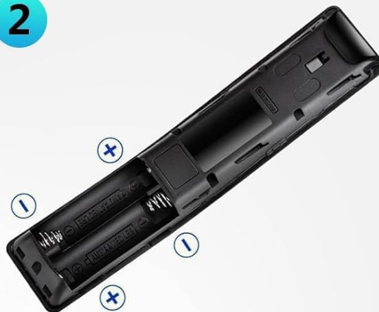
Distinguish the positive and negative electrodes of the battery
