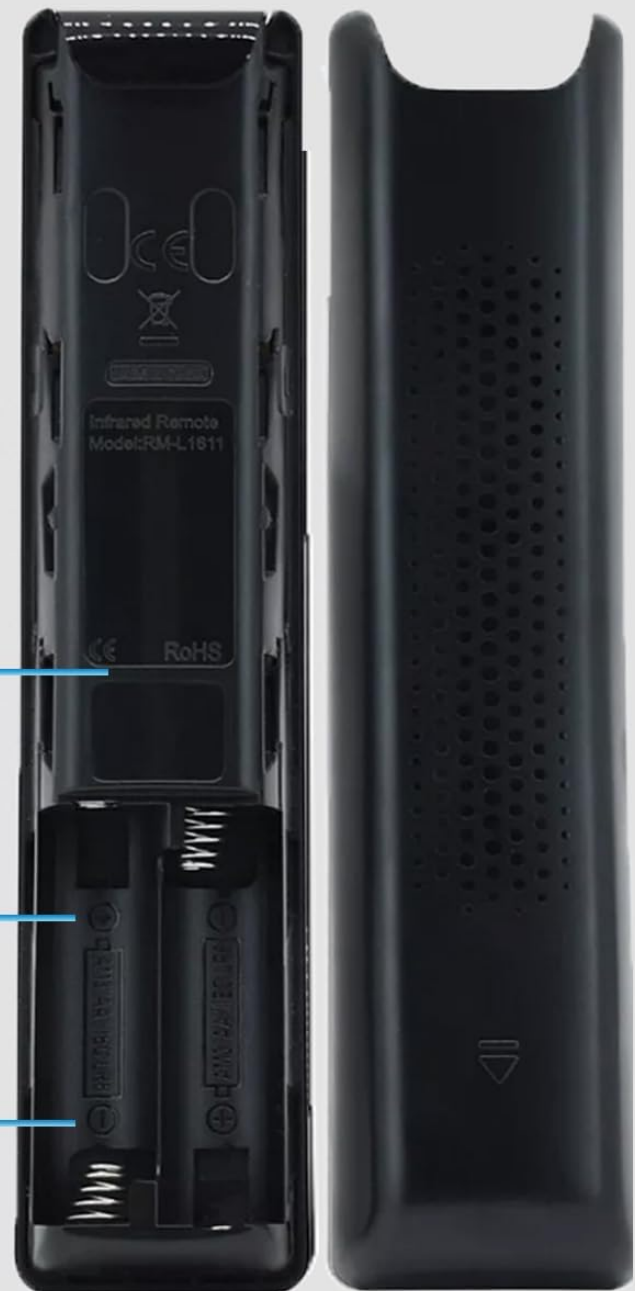
Figure 1: Battery compartment and correct battery orientation.
