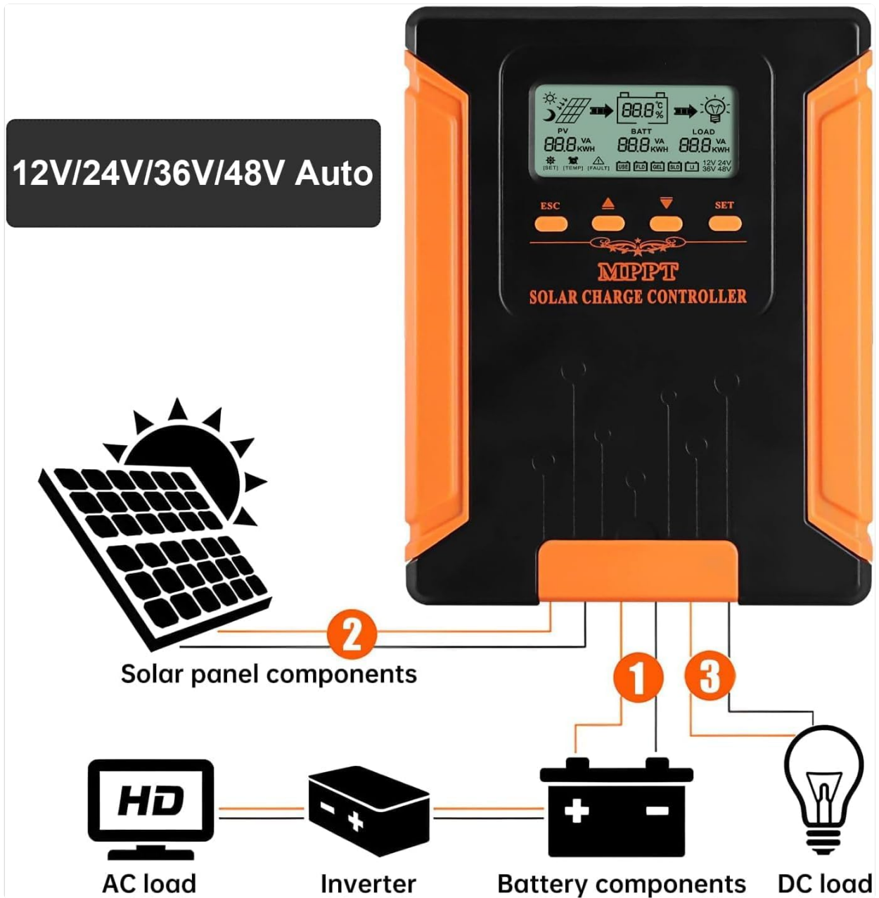
Figure 6: Connection diagram illustrating the proper wiring sequence for solar panels, battery, and DC load.
