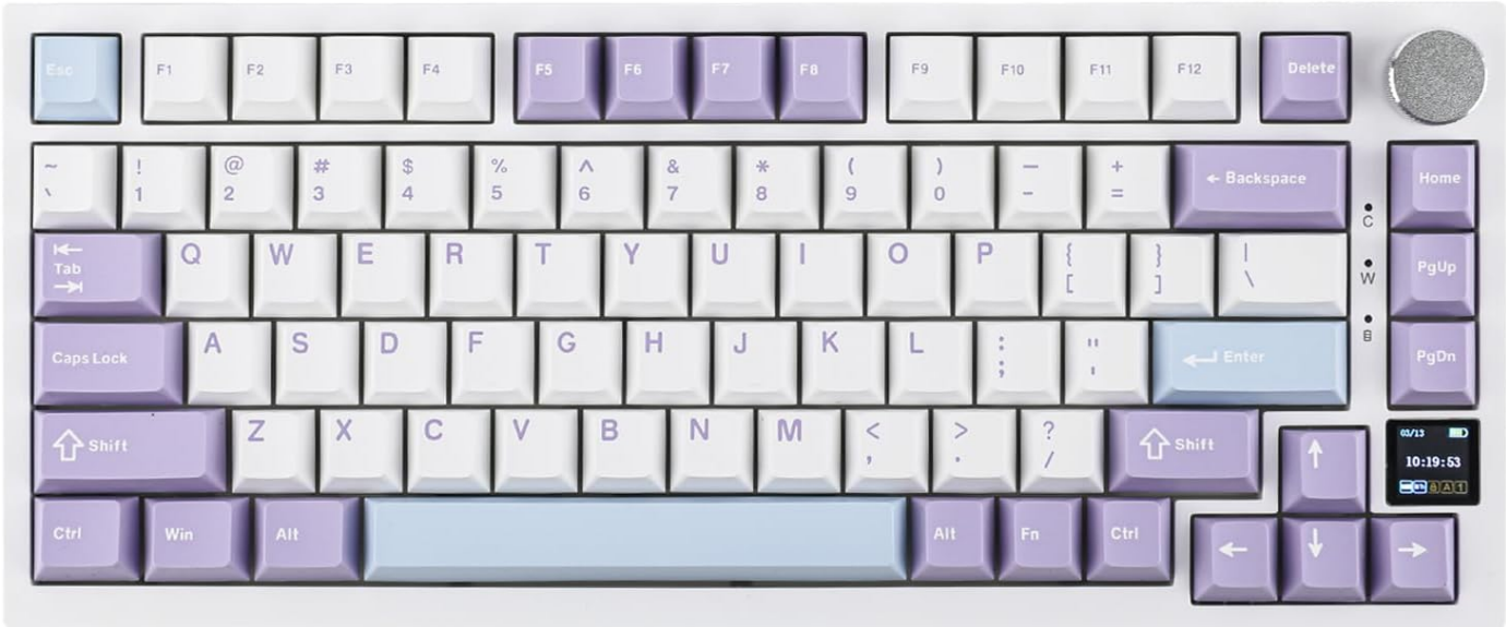
Image: Top-down view of the EPOMAKER Ajazz AK820 Pro keyboard, showcasing its 75% layout, purple and white keycaps, and the smart display and knob.
