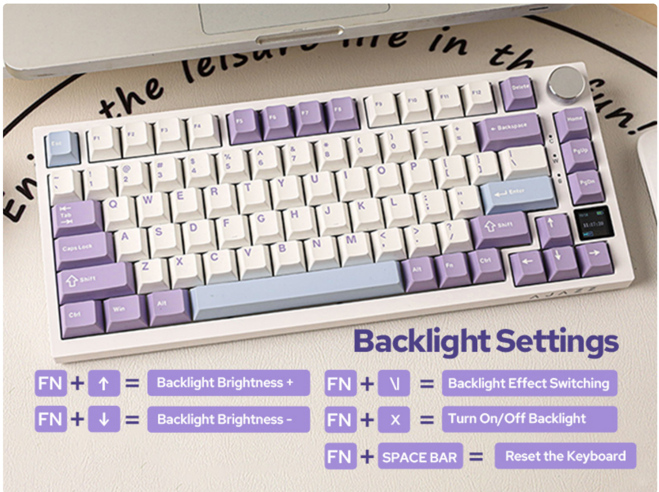
Image: Visual guide showing the function key combinations for adjusting backlight settings.
