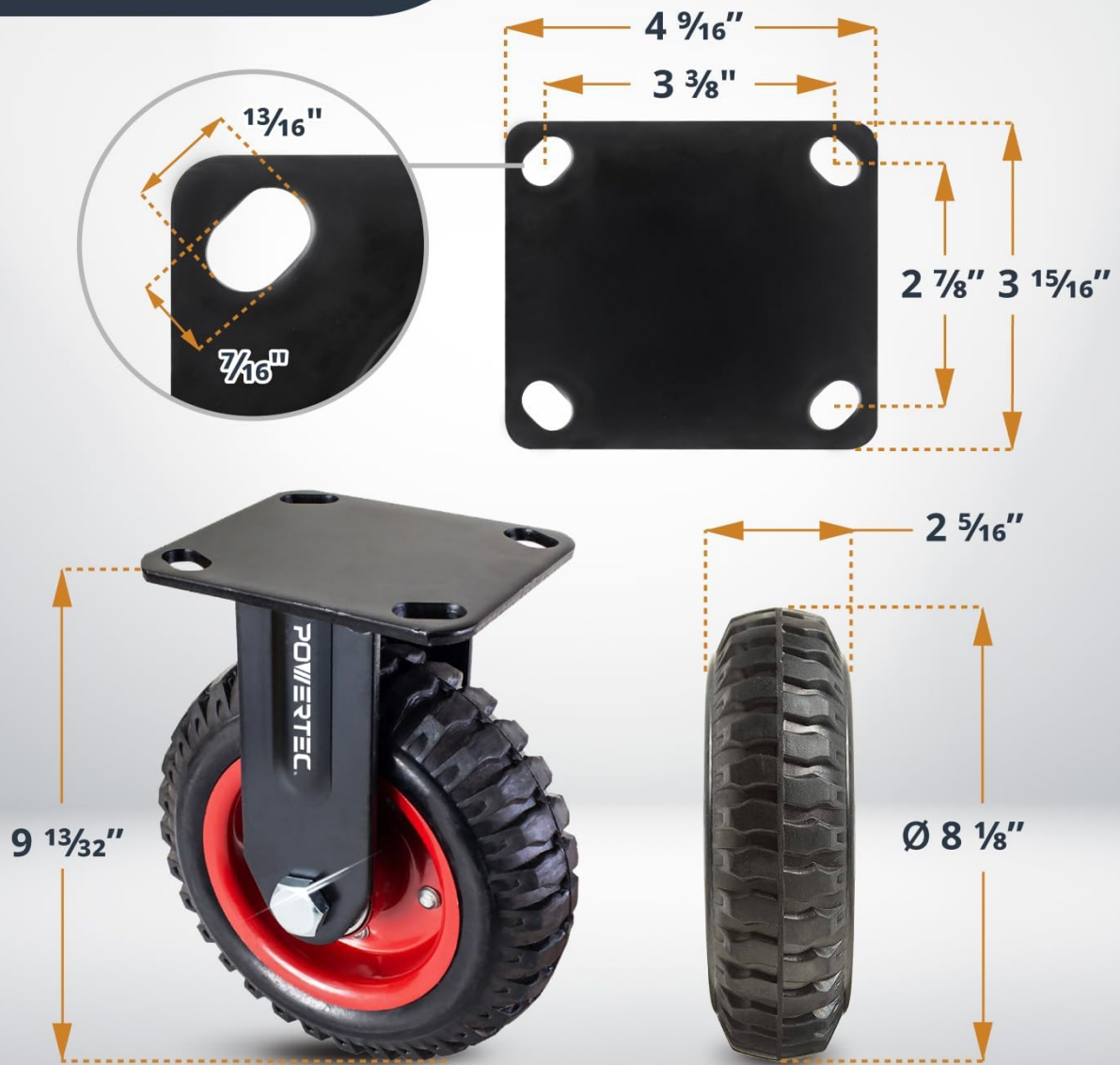
Figure 2: Fixed Caster Dimensions. This image provides detailed measurements for the fixed caster wheel and its mounting plate, showing plate size, hole spacing, wheel diameter, and overall height.
