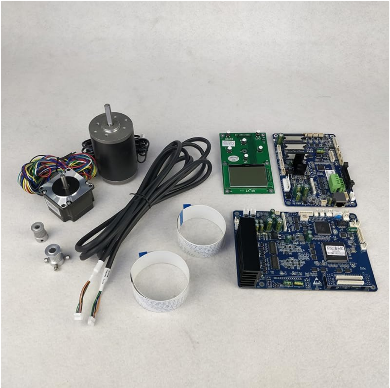
Image 3.2: Another perspective of the Senyang Board DX5 Conversion Kit. This view highlights the different types of cables and the two main circuit boards, along with the motors, providing a comprehensive look at the included hardware.
