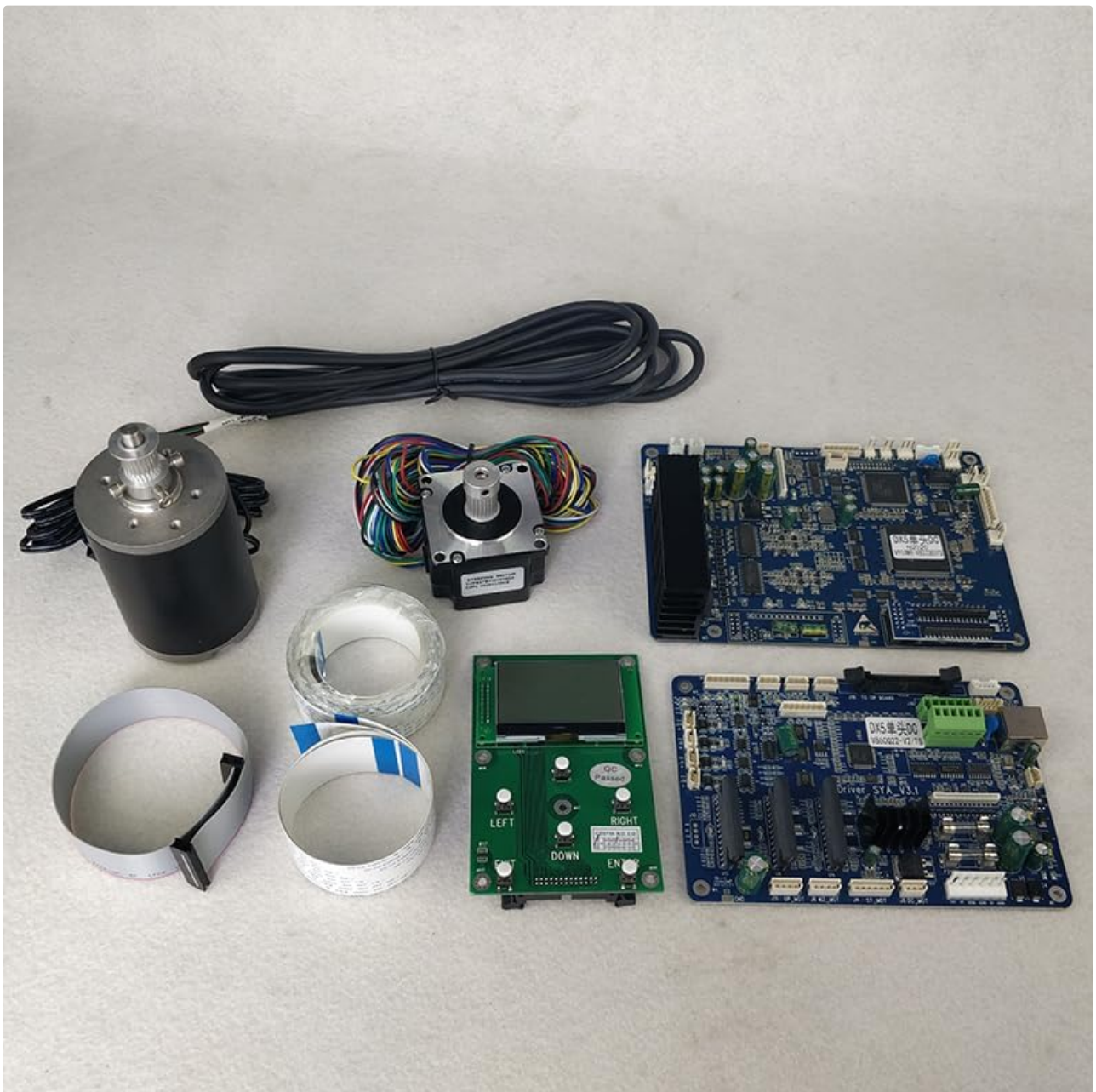
Image 3.1: Overview of the Senyang Board DX5 Conversion Kit components. This image displays the main control boards, stepper motors, various cables, and a small display panel, which are typical parts of the conversion kit.
