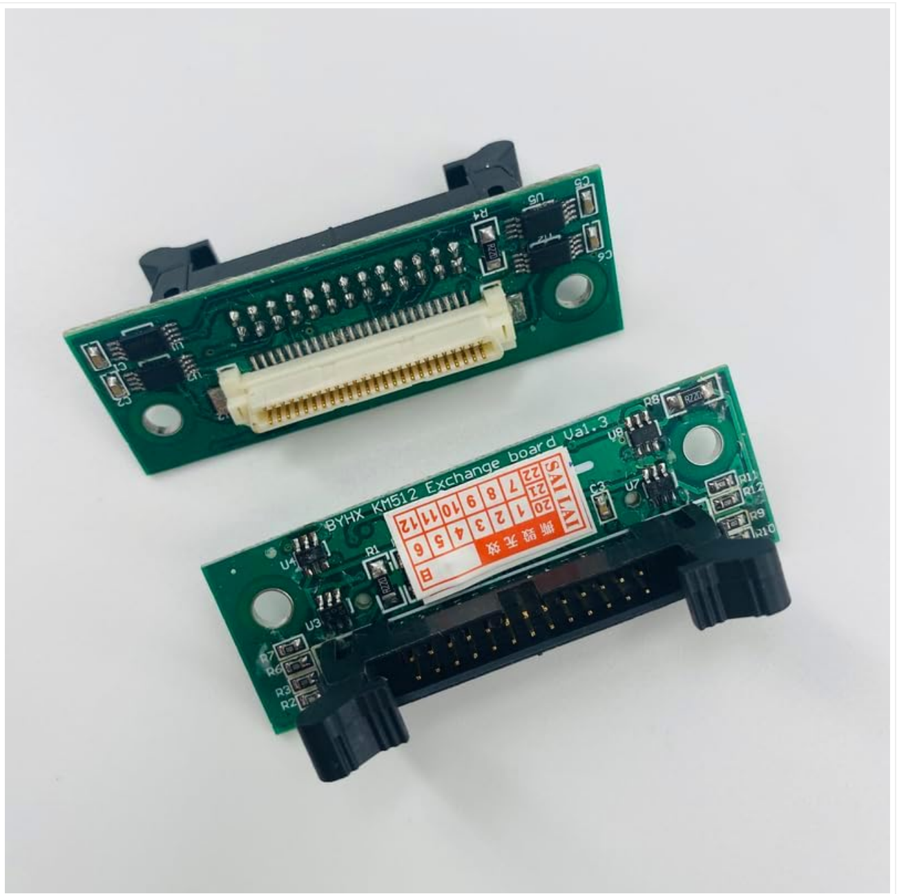
Figure 1: Front and back view of the BYHX KM512 Printhead Transfer Board VB1.4 Adapter Head Connector.
