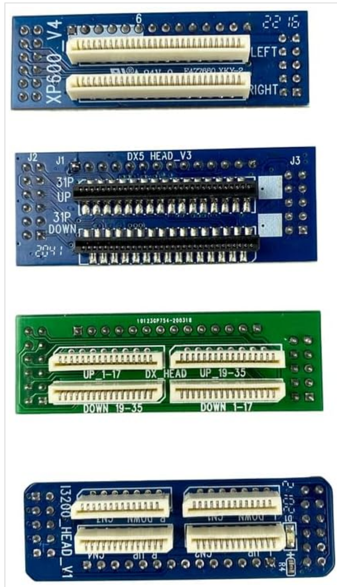
Figure 2: Comparison of various Senyang Headboard Connect Cards. This image shows four different headboard connector boards, each designed for a specific print head type: XP600, DX5, DX, and I3200. The I3200 board is at the bottom, identical to Figure 1, highlighting the importance of selecting the correct part for your printer model.
