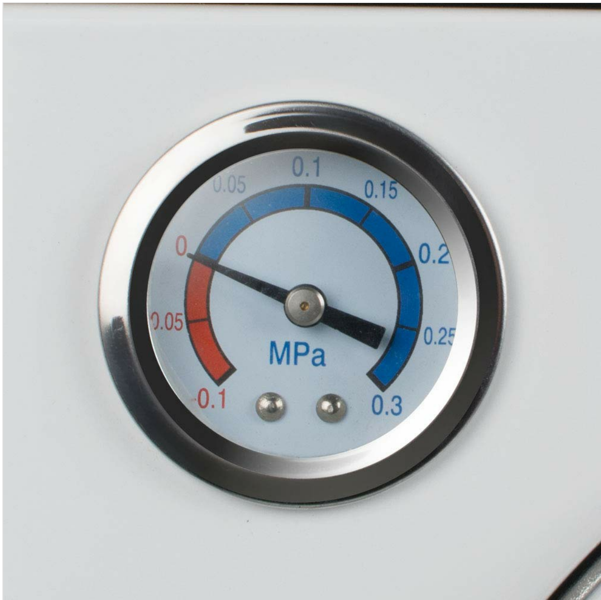
Figure 3.5: Close-up view of the autoclave's analog pressure gauge, clearly marked in MPa, with a needle indicating the current pressure level within the chamber.
