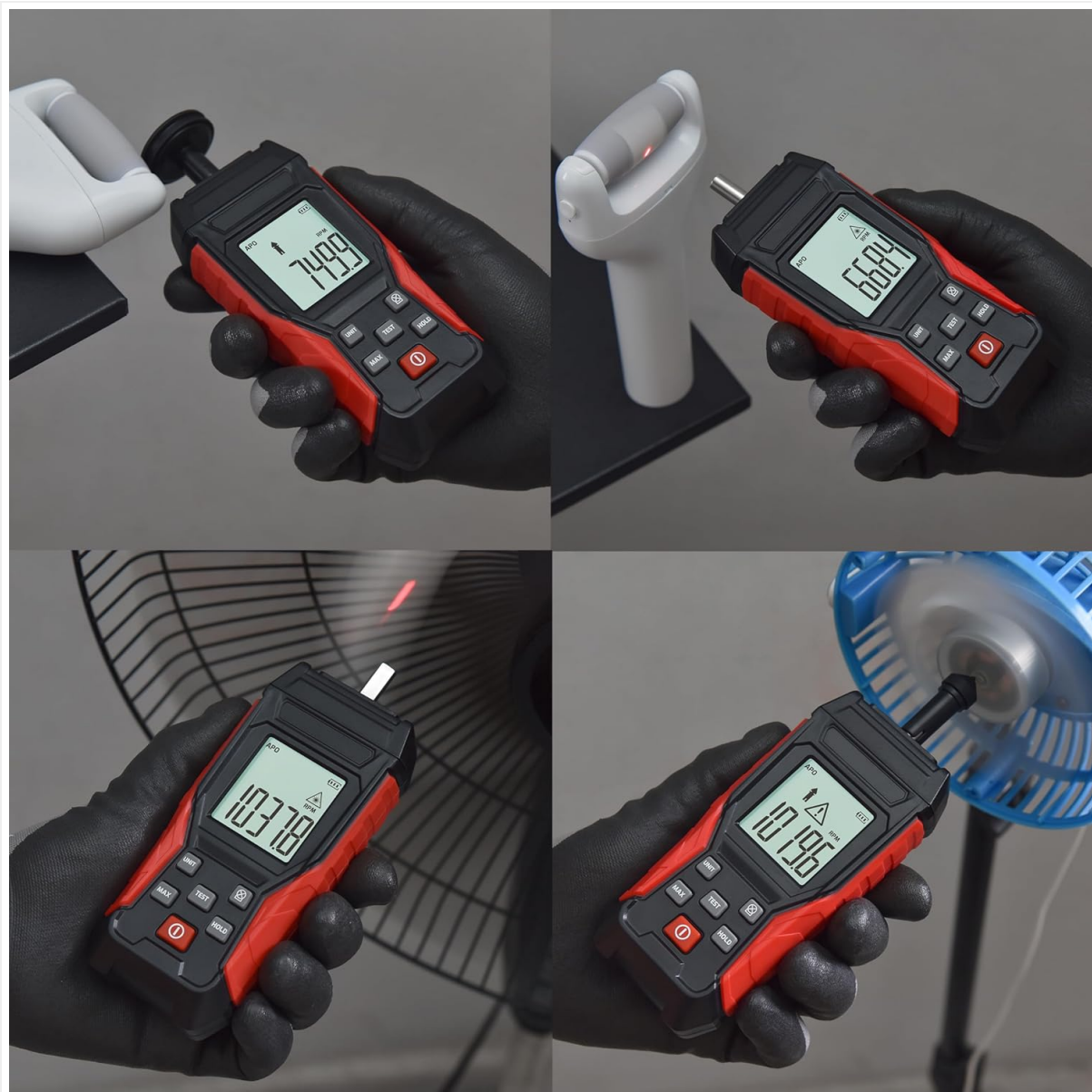
Figure 4.1: Examples of the HFS TMT-JP meter being used for both contact and non-contact measurements on different rotating objects.
