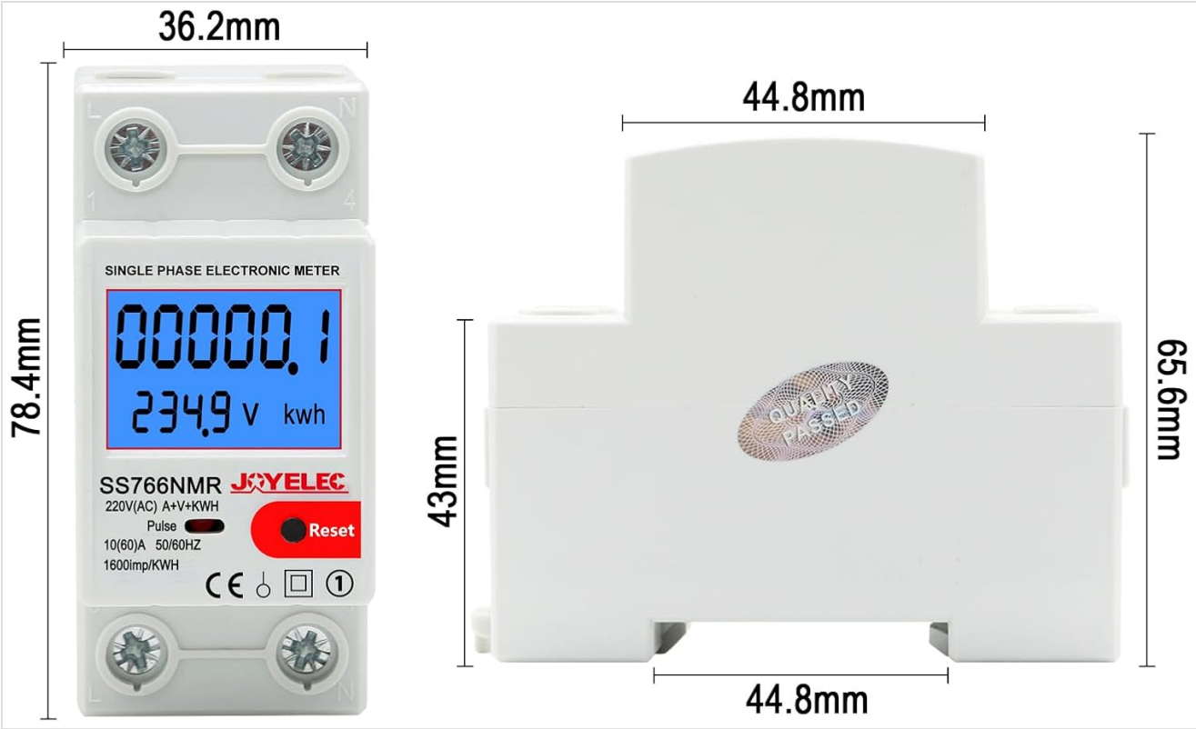
Image 2: Dimensional drawing of the energy meter. The front face measures approximately 36.2mm wide and 78.4mm high. The side view shows a depth of 44.8mm and a total height of 65.6mm, with the DIN rail clip extending 43mm from the top surface.
