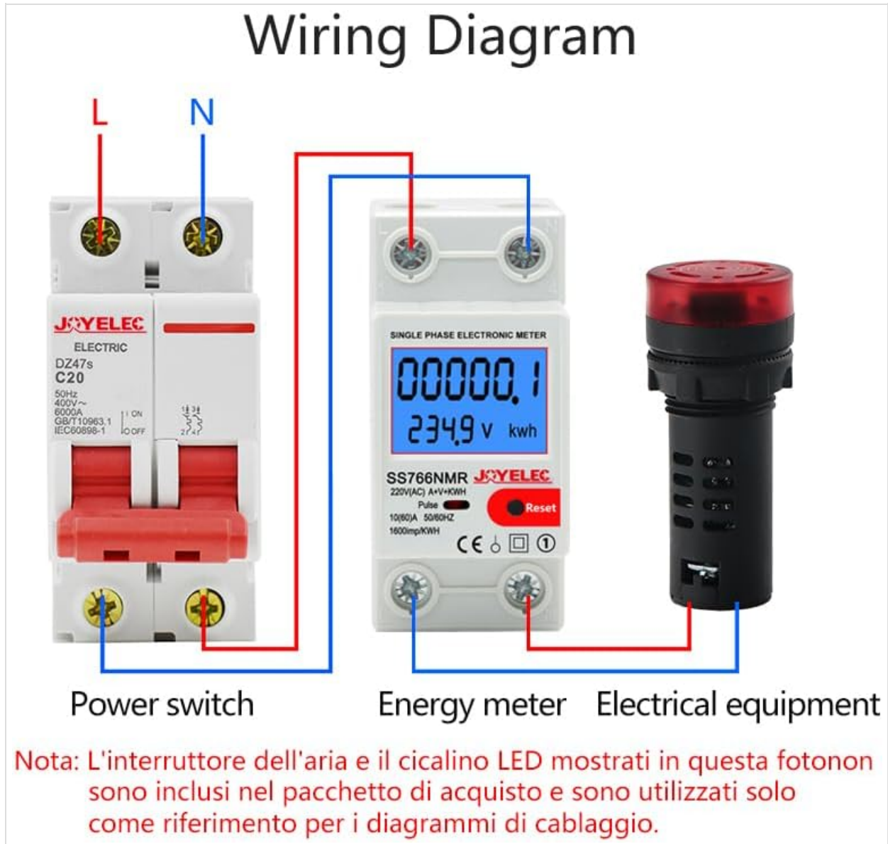
Image 4: Wiring diagram illustrating the connection of the JOYELEC SS766NMR energy meter. The incoming Live (L) and Neutral (N) wires connect to the top terminals. The outgoing Live (L) and Neutral (N) wires connect to the bottom terminals, leading to the electrical equipment. A power switch is shown upstream of the meter for reference, though not included with the meter.
