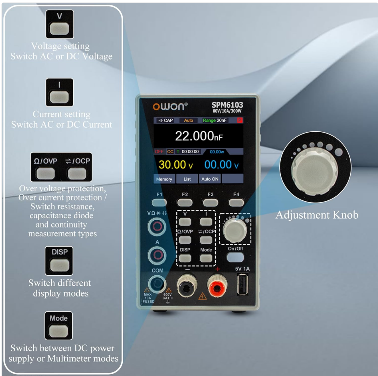
Figure 2: Detailed Front Panel Controls. This image highlights the functions of various controls: Voltage setting, Current setting, Over voltage/current protection, resistance, capacitance, diode, and continuity measurement types, Switch different display modes, Mode button for switching between DC power supply or Multimeter modes, and the Adjustment Knob.
