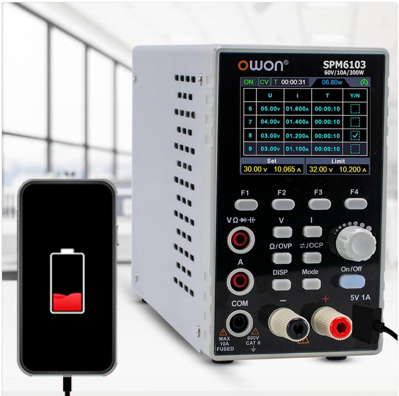
Figure 4: List Waveform Editing and Charging Function. This image illustrates the device's capability to perform timed output sequences and charge external devices via the 5V USB port.
