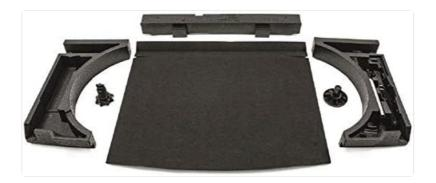
This image displays all the essential components included in the Skoda spare wheel installation kit. Visible are the two large, curved polystyrene boxes designed to fit around the spare wheel, a flat floor covering, and a smaller rectangular piece which is likely the fastening matrix or part of the toolbox. These components are designed to organize and secure the spare wheel and associated tools within the vehicle's trunk.
