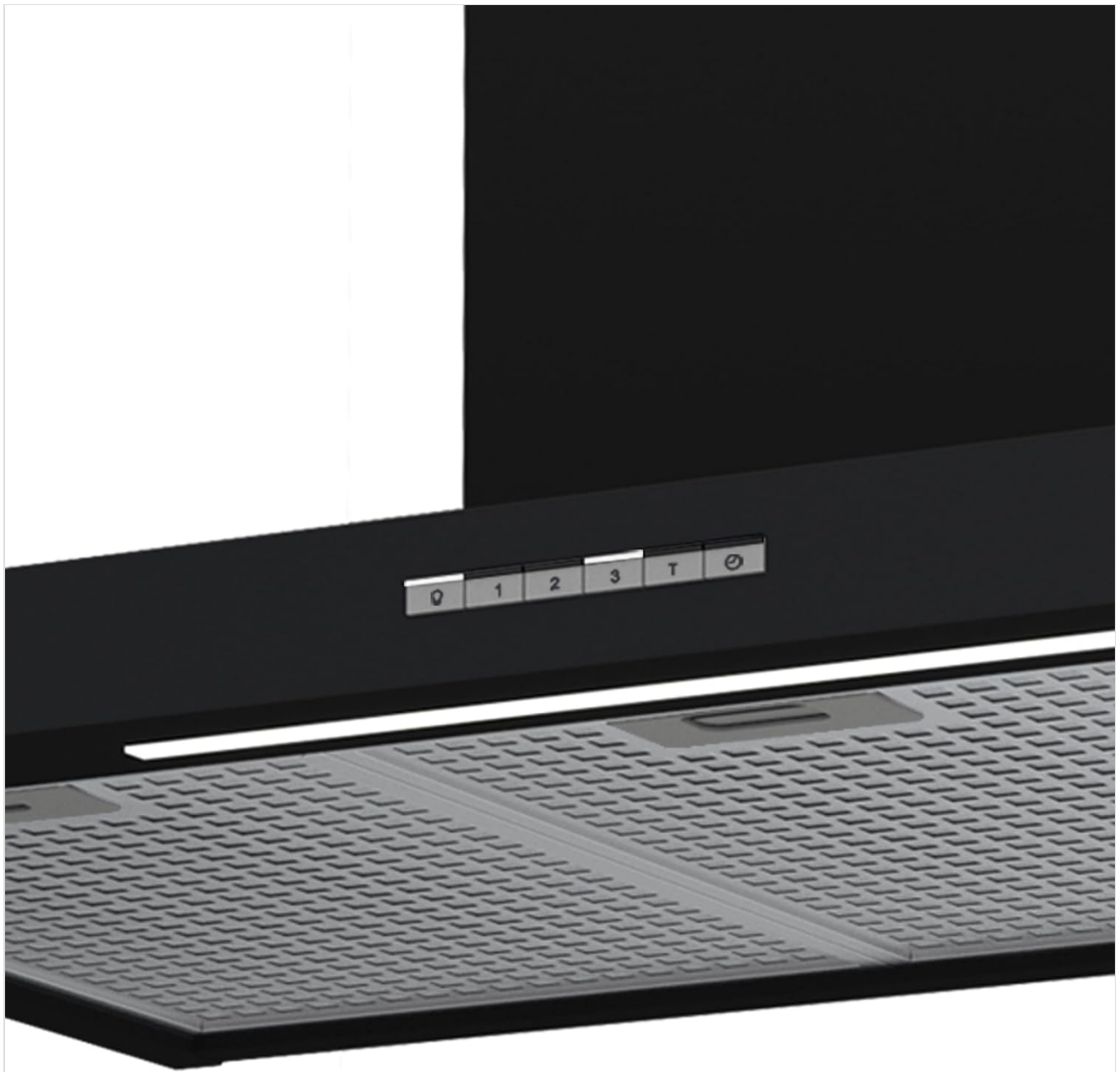
Image: Close-up view of the electronic control panel on the CATA Sygma 9010 BK hood, showing touch buttons for light, three extraction speeds, a Turbo function, and a timer.
