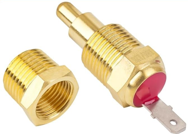
3/8" NPT Pipe Thread with 1/2" Adapter 185 Degrees On 175 Degrees off
