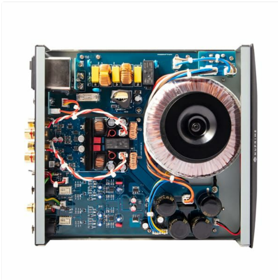
Figure 6.1: Internal view of the NuPrime STA-9X. This image provides a glimpse into the amplifier's internal components, including the high-efficiency toroidal transformer and the meticulously designed circuit board.
