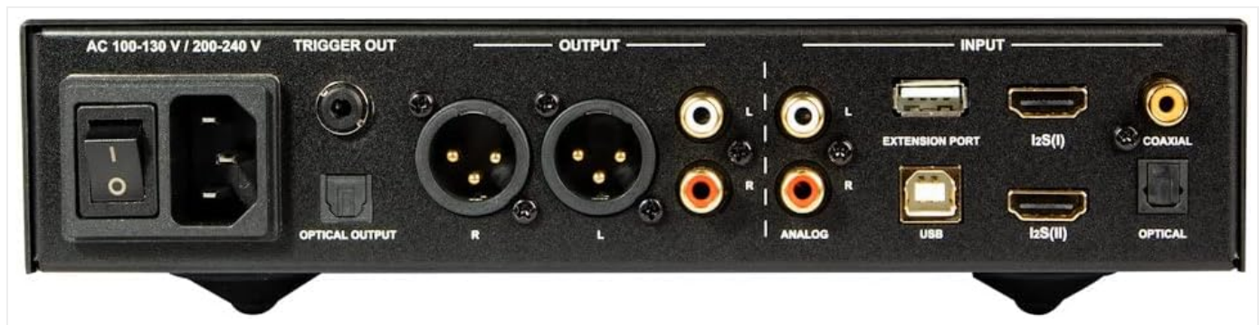
Figure 3: Rear panel of the NuPrime DAC-9X, illustrating available connections.
