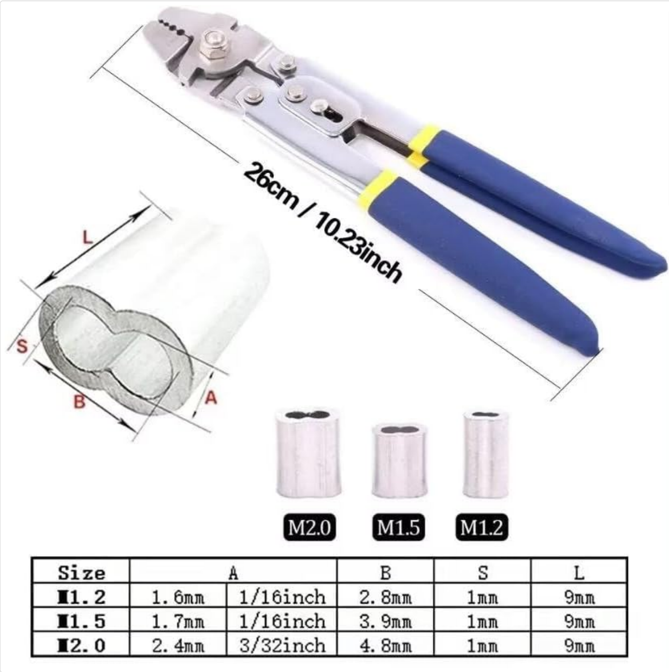
Figure 9: Detailed diagram of double barrel ferrules with size specifications (M1.2, M1.5, M2.0) and a table of their dimensions (A, B, S, L).
