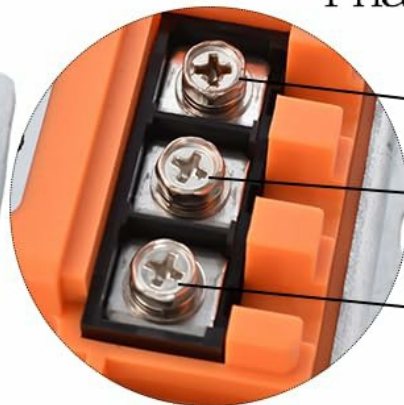
Image 2.3.4: Close-up of battery and phase wire terminals.
