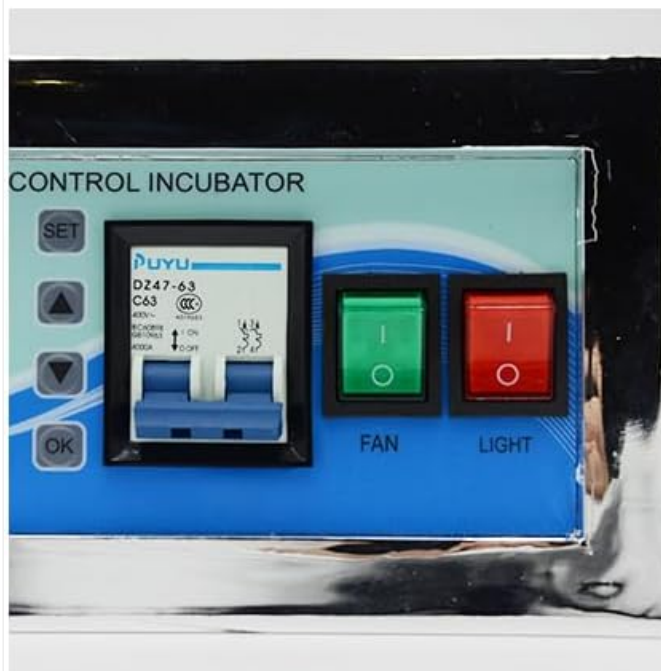
Figure 4.4: Key features of the XM-18D controller. It offers real-time measurement and control of temperature and humidity, along with button touch operation for simple and convenient use.
