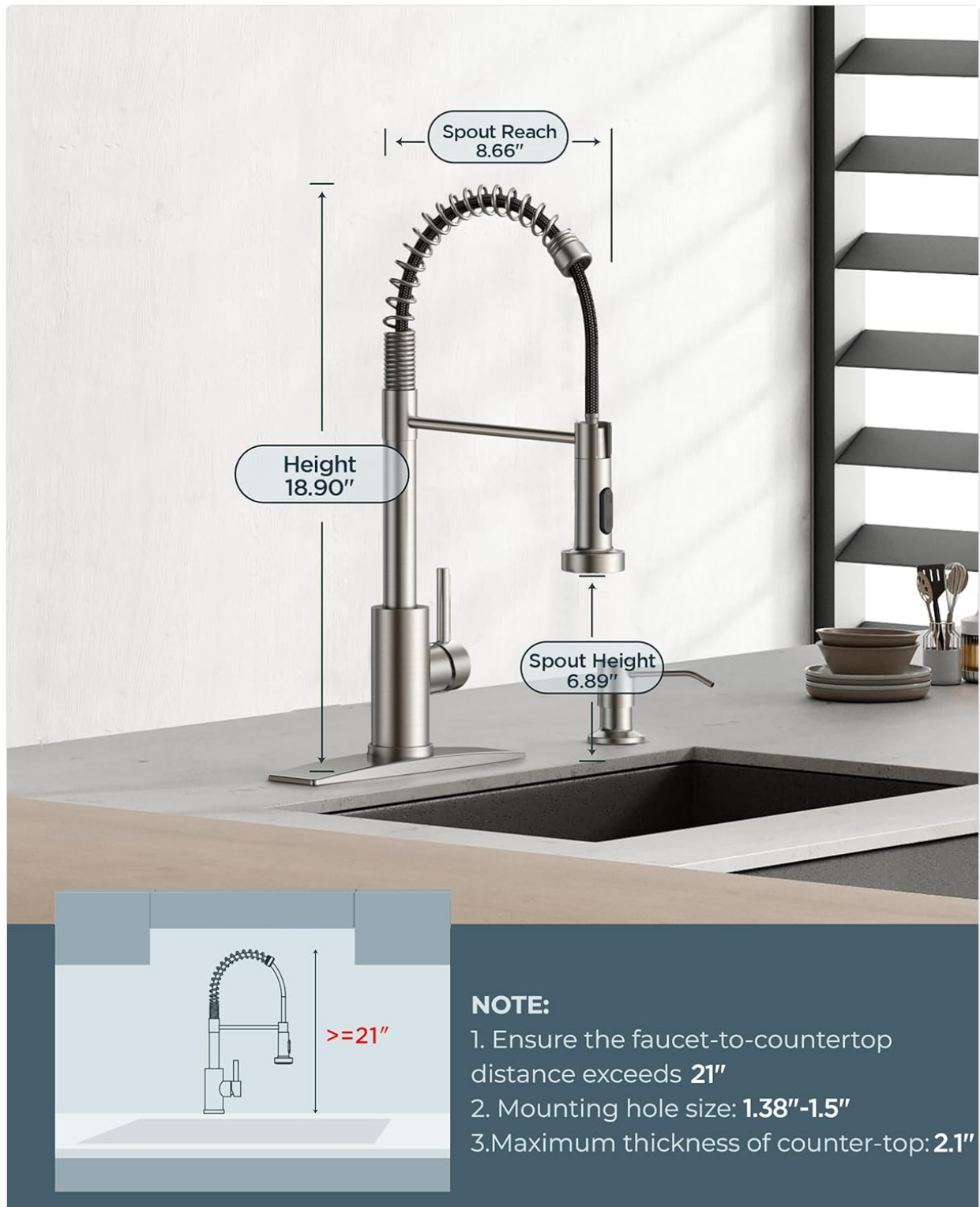
Image: Faucet dimensions and installation notes for proper fit.
