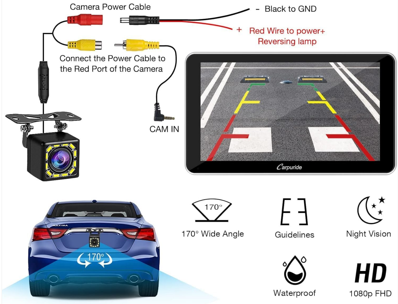
Figure 5.2: Rear View Camera Wiring Diagram. This diagram provides a visual guide for connecting the rear camera to the main unit and the vehicle's power system, ensuring automatic activation upon reversing.
