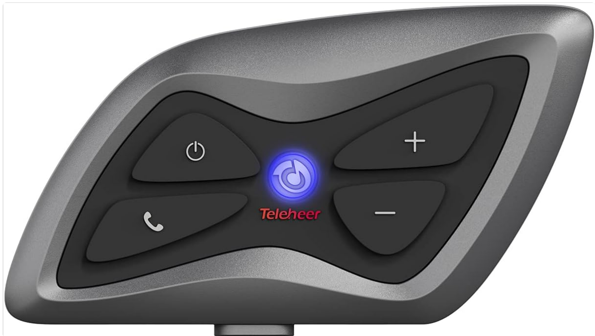
Image 1: Front view of the Teleheer T6 Plus intercom unit. It features a sleek, dark grey casing with five distinct buttons. From left to right, top row: Power button (circle with vertical line), Intercom button (glowing blue circle with a 'd' like symbol), Plus button (+). Bottom row: Phone button (curved phone icon), Minus button (-). The 'Teleheer' logo is visible below the intercom button.
