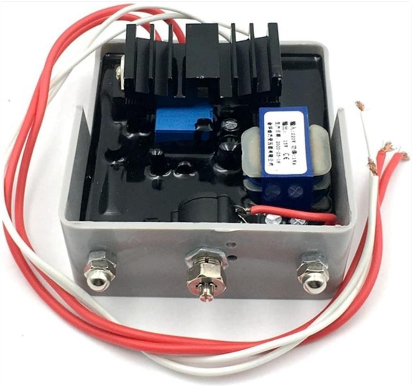
Figure 4: An alternative angled view of the GB170C AVR, providing a comprehensive look at its assembled state, including the protective casing, internal components, and wiring leads.
