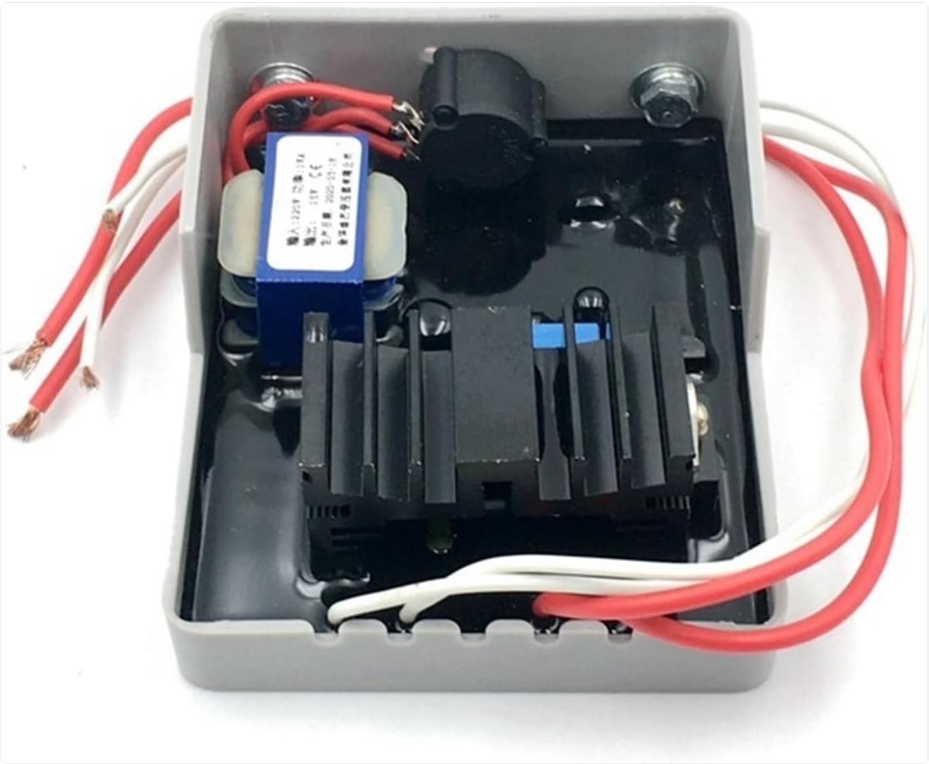
Figure 1: Top-down view of the GB170C AVR, showing the internal transformer, heat sink, and wiring terminals. The red and white wires are visible, indicating connections for the generator.
