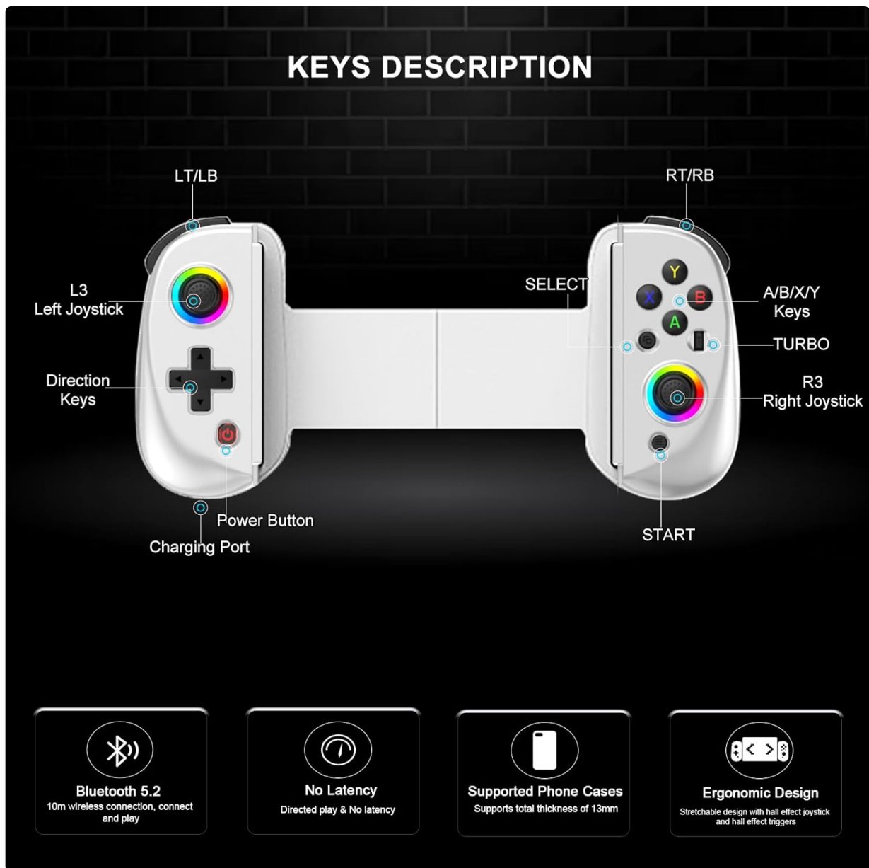
Image: Overview of the arVin D8 controller, highlighting the Power Button, Charging Port, L3 (Left Joystick), Direction Keys, LT/LB, SELECT, A/B/X/Y Keys, TURBO, R3 (Right Joystick), and START buttons.
