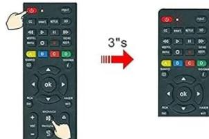
**Step.2** Input your 3 digit TV CODE from code list. If the code is right, the LED light will go off. If the code is wrong, the LED light will still be on. If this happens, try to enter the code again as there may have been an error the first time. (If the TV not
