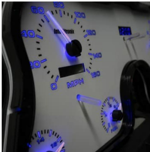
Image: A detailed view of the speedometer, featuring blue backlighting, an analog needle indicating speed in miles per hour, and a digital display for the odometer.
