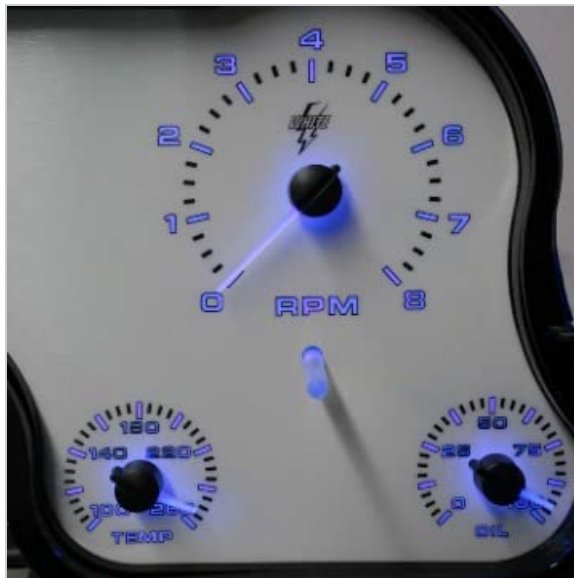
Image: A close-up of the tachometer, illuminated in blue, displaying engine RPM. Below it are smaller gauges for water temperature and oil pressure.
