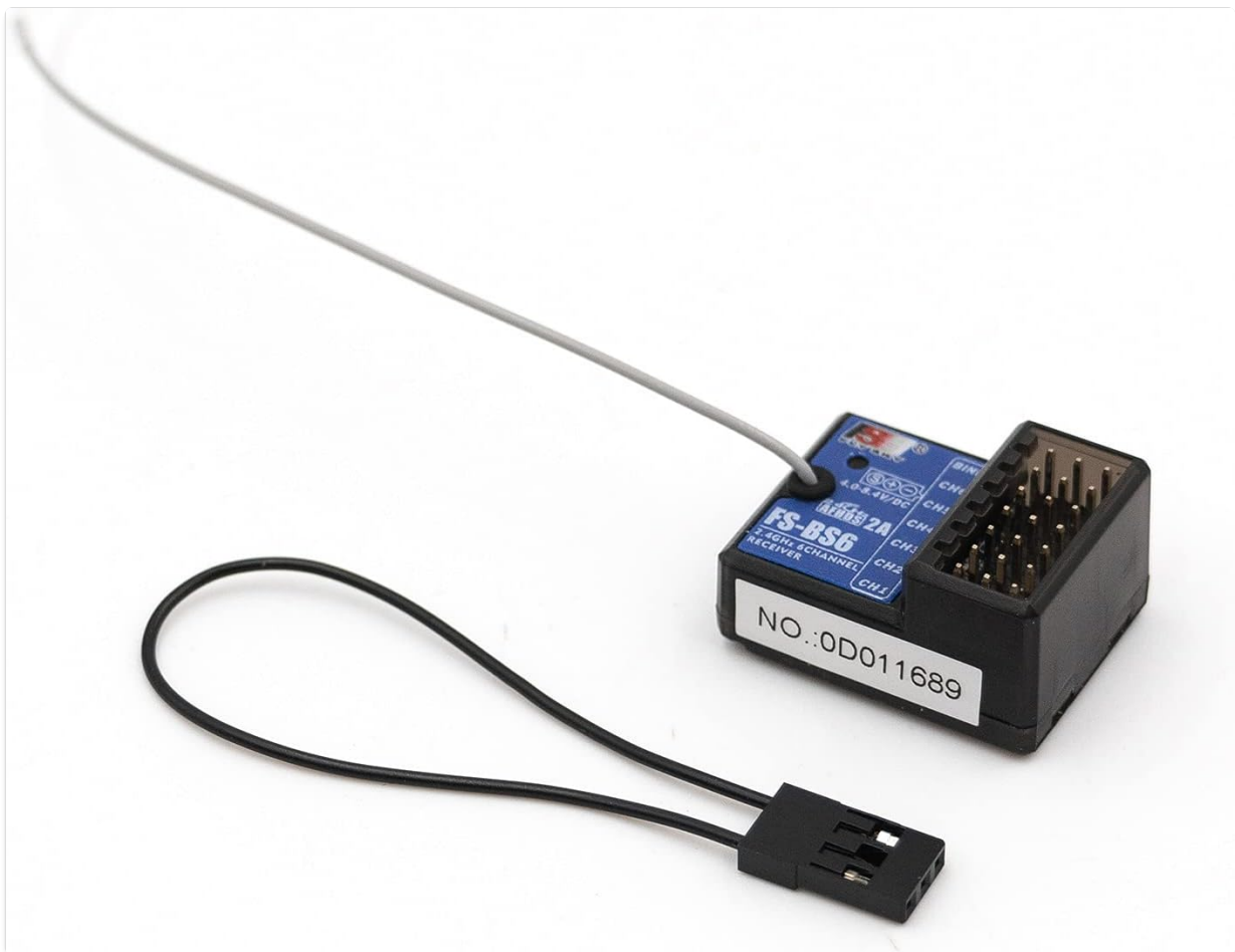
Image 4.2: FS-BS6 receiver with bind plug and antenna.
