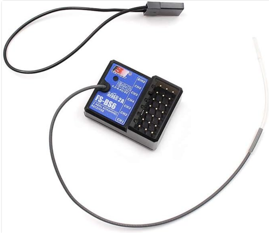
Image 4.1: FS-BS6 receiver with bind plug inserted.
