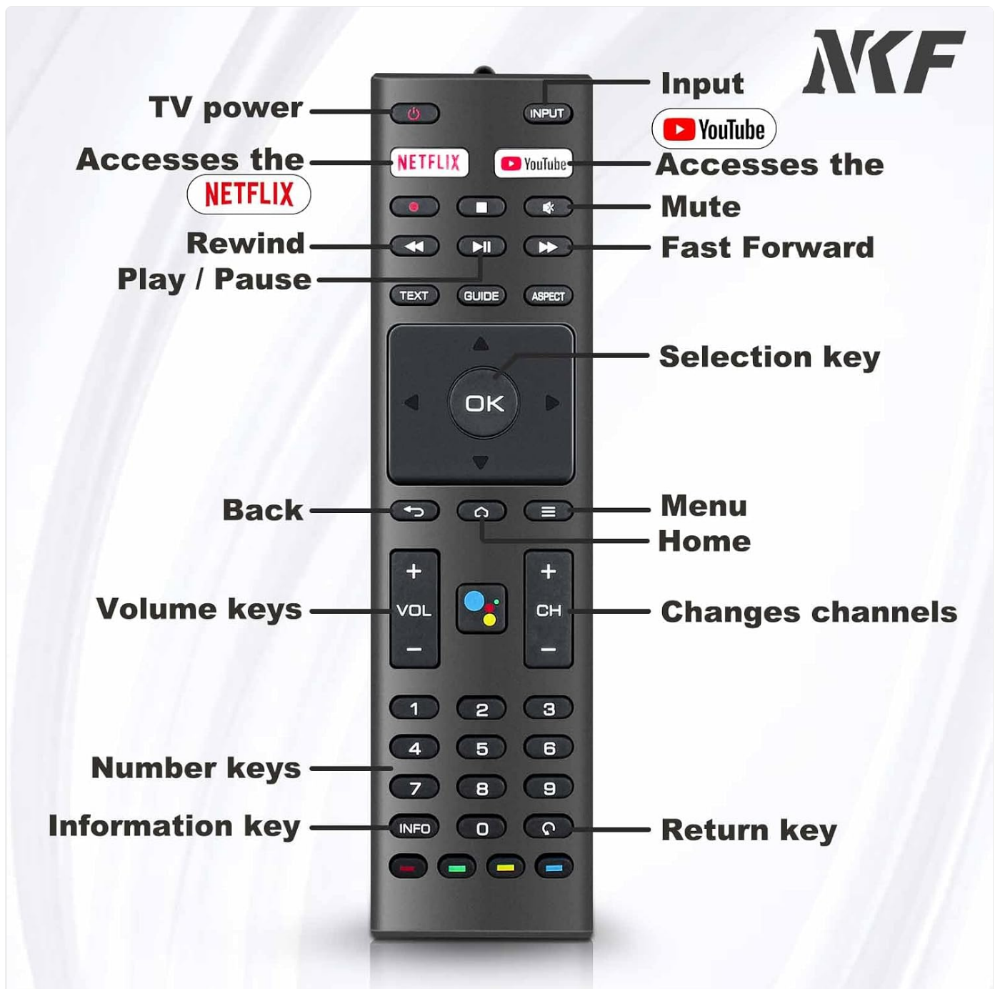
Figure 2: Labeled diagram of the RM-C3329 remote control buttons and their functions.
