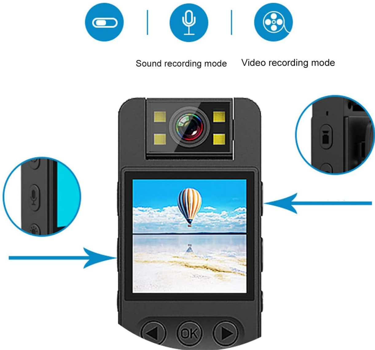
Figure 4.1: Simple operation with dedicated buttons for recording modes.
