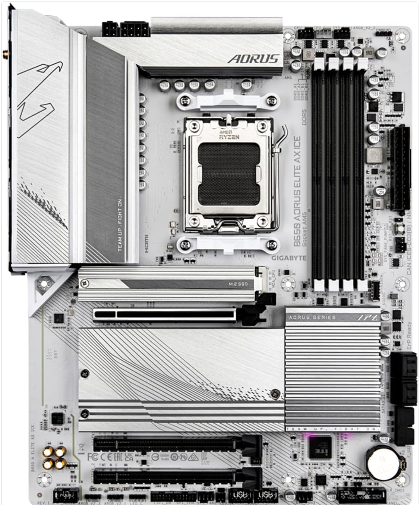
Figure 2.2: Top-down view showing the AM5 CPU socket.
