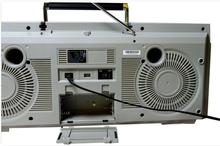
Figure 4.3: Rear view of the Soundmaster SCD1980SI Boombox, displaying the power input, battery compartment, and bass reflex ports.
