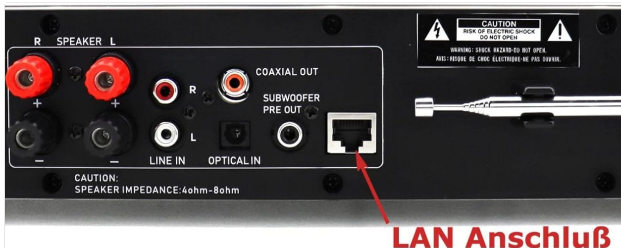
Image 3.1: Rear panel connections, including LAN port.
