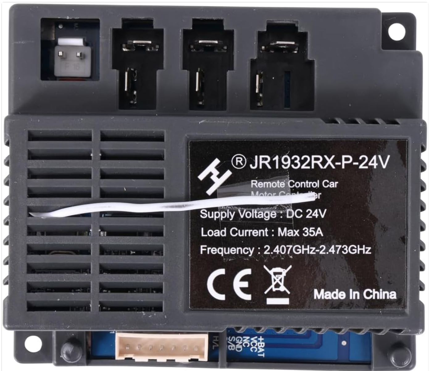
Image 2: A detailed view of the SHENGLE JR1932RX-P-24V control box, highlighting its various ports and the label with electrical specifications. This image is useful for identifying connection points during installation.
