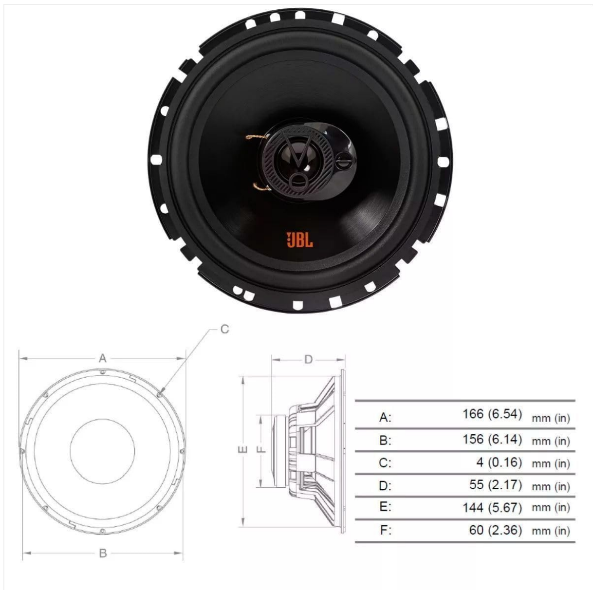
Image: Technical diagram illustrating the dimensions of the JBL 6TRFX55 speaker for accurate mounting and fitment.
