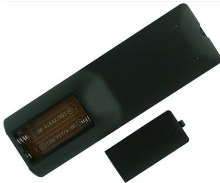
This image shows the back of the remote control with the battery cover removed, revealing the two slots for AAA batteries.
