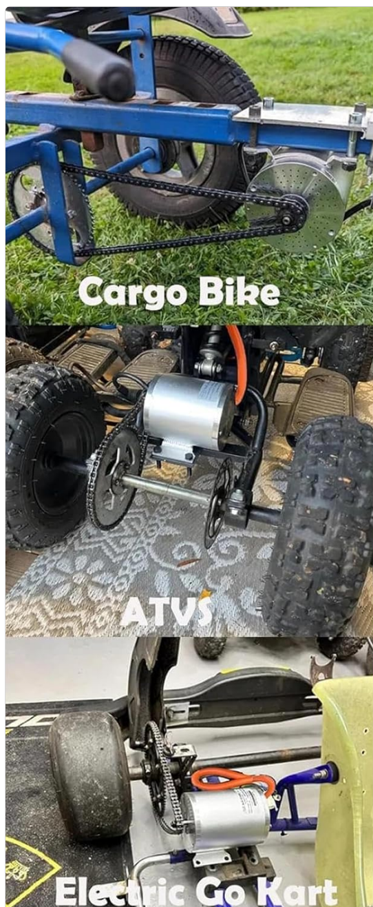
Figure 9.1: Examples of vehicles compatible with the Kunray motor kit, including cargo bikes, ATVs, and electric go-karts.
