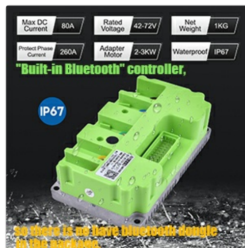
Figure 5.4: The controller's IP67 waterproof design.
