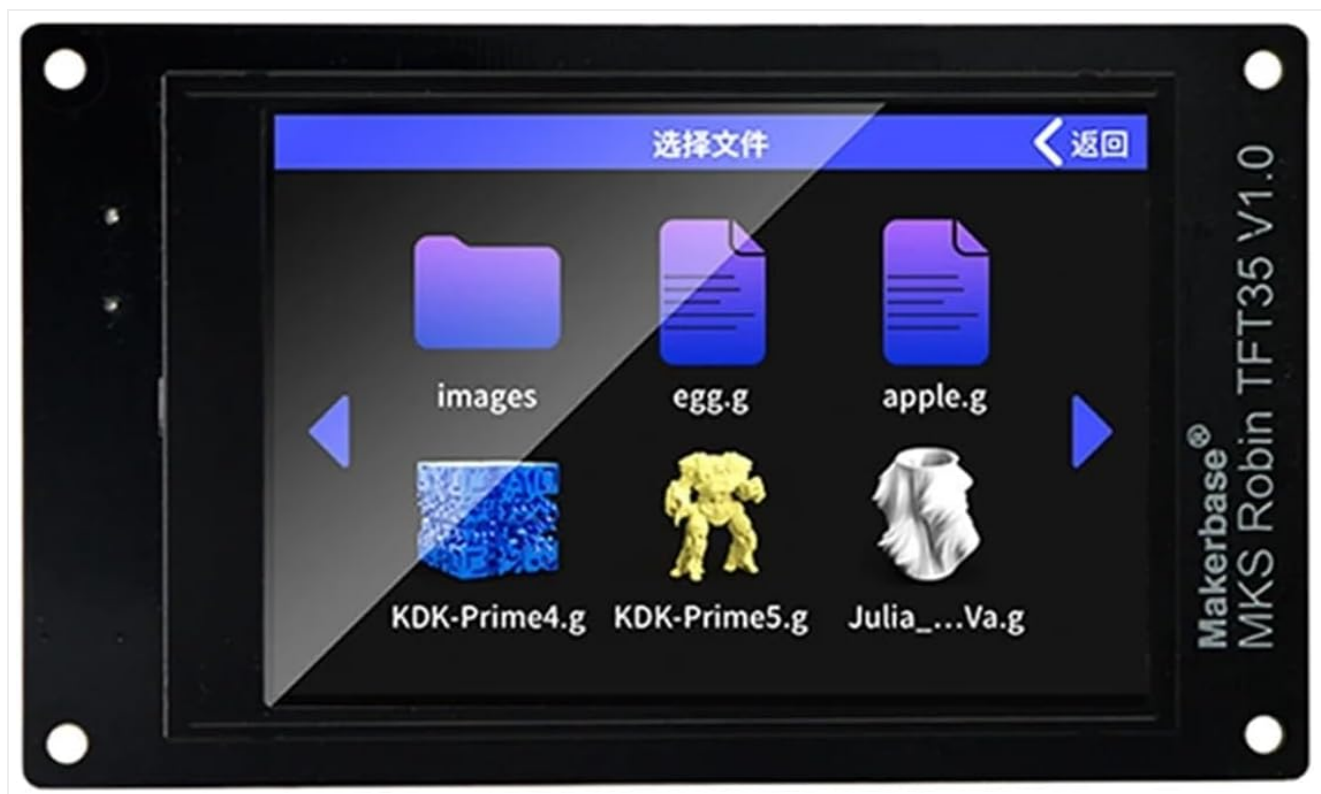
Figure 4: MKS Robin TFT35 V1.0 Touch Screen displaying file selection interface. This image shows the user interface of the touch screen, typically used for selecting print files and controlling the 3D printer.
