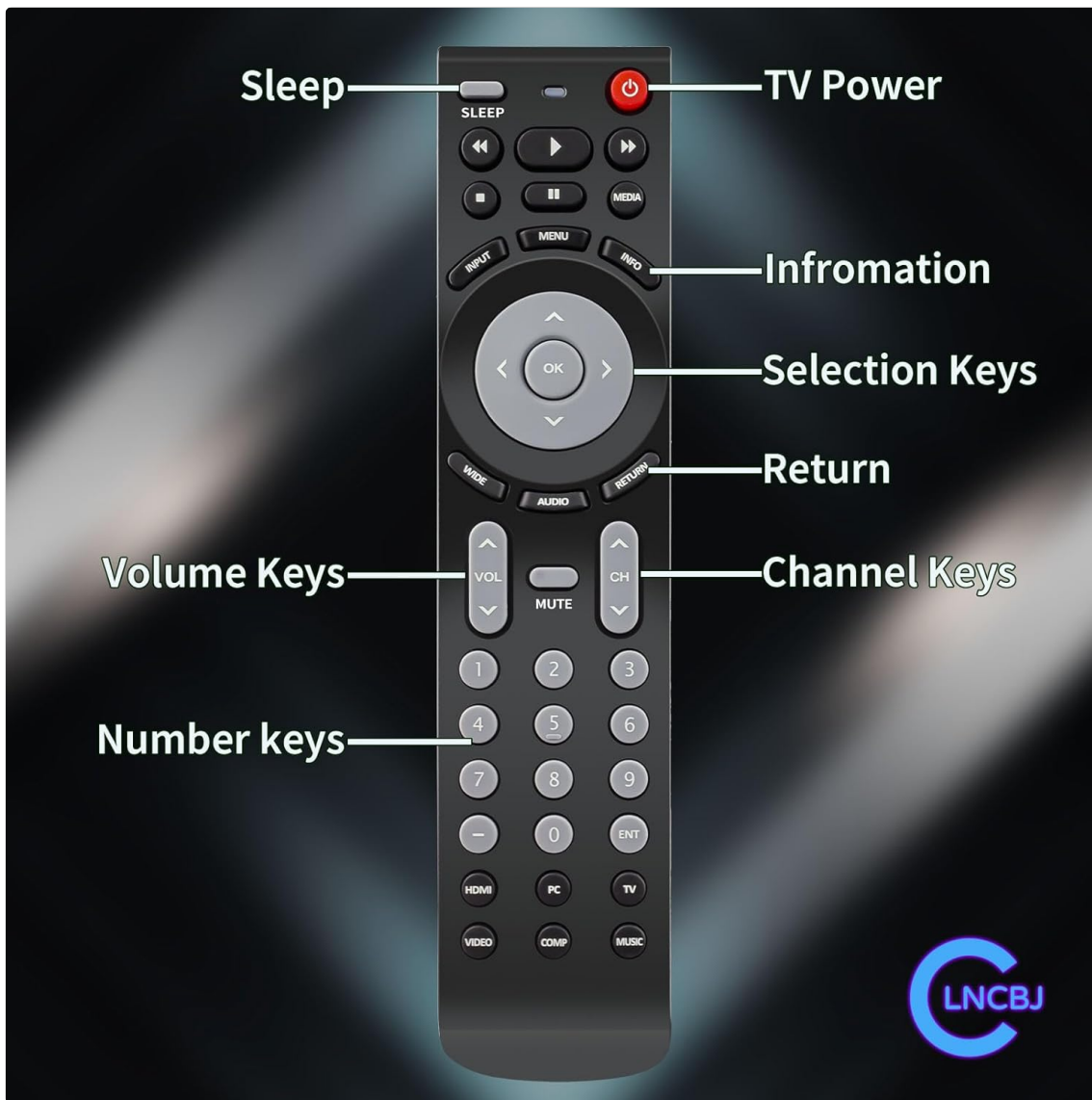
Image 3.1: Diagram illustrating the main buttons and their functions on the RMT-JR01 remote control.
