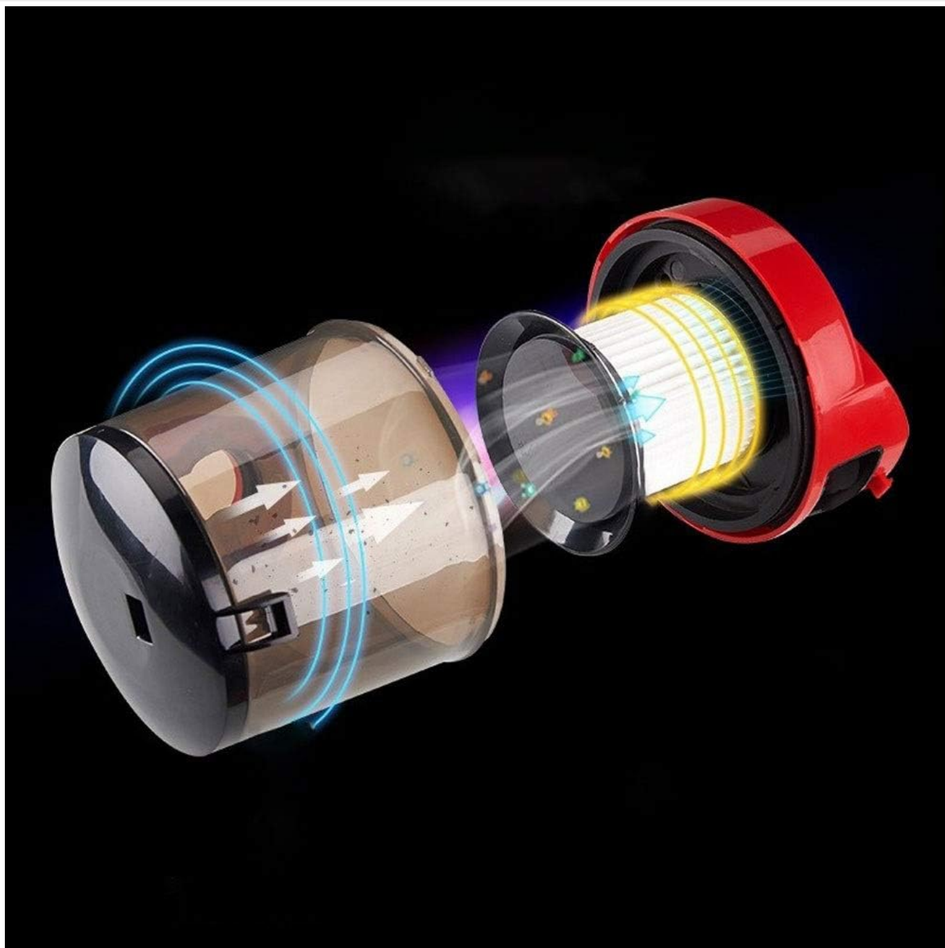
Figure 5.1: An exploded view illustrating the internal components of the vacuum's dust collection system, specifically highlighting the dust bin and the multi-layered filter. Blue arrows indicate the airflow path, showing how air passes through the filter to separate dust particles, ensuring clean exhaust air.
