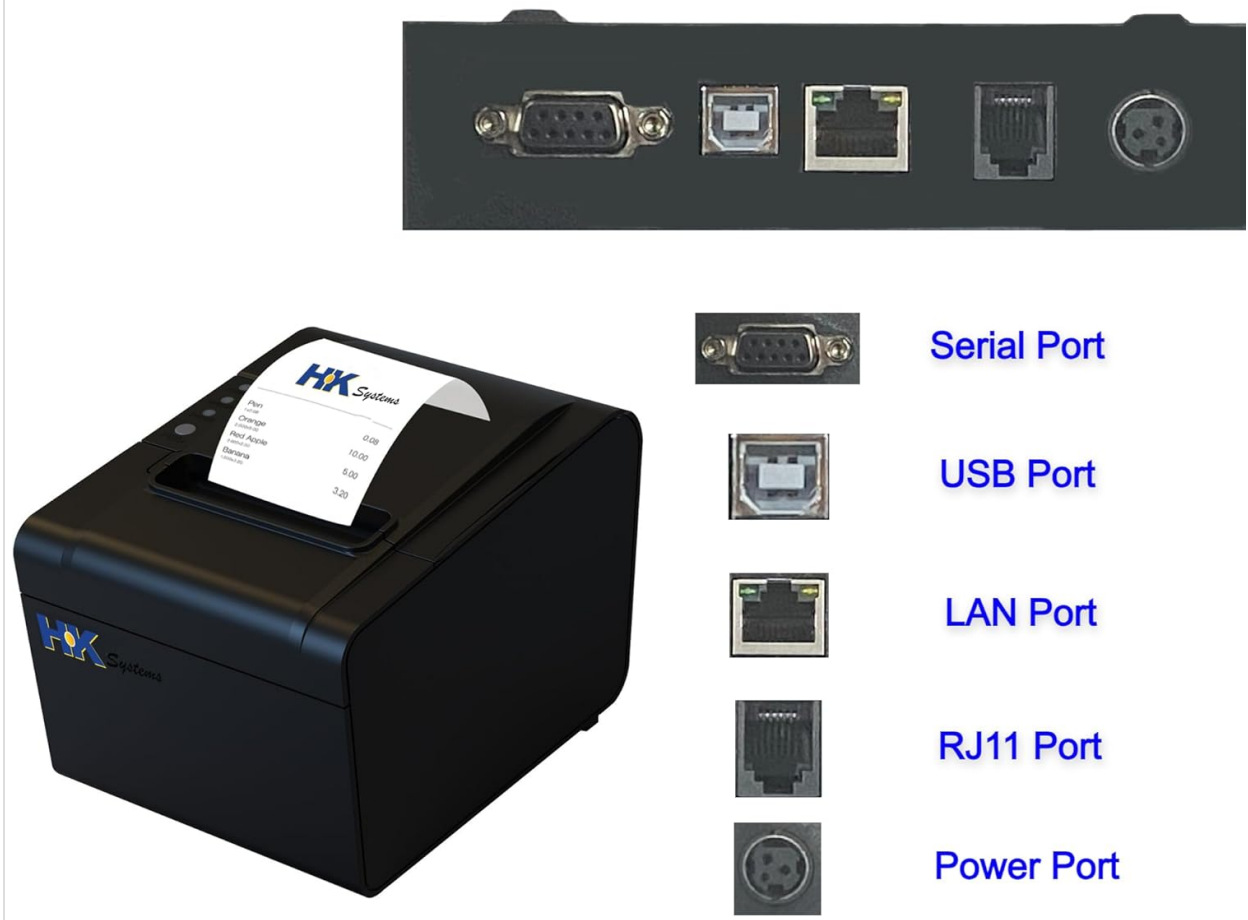
Figure 3: Rear view of the printer highlighting available interfaces.
