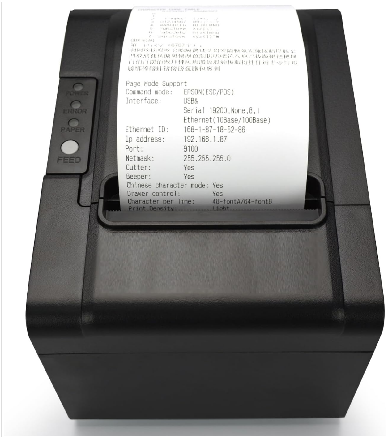
Figure 4: Printer displaying a self-test receipt with configuration details.
