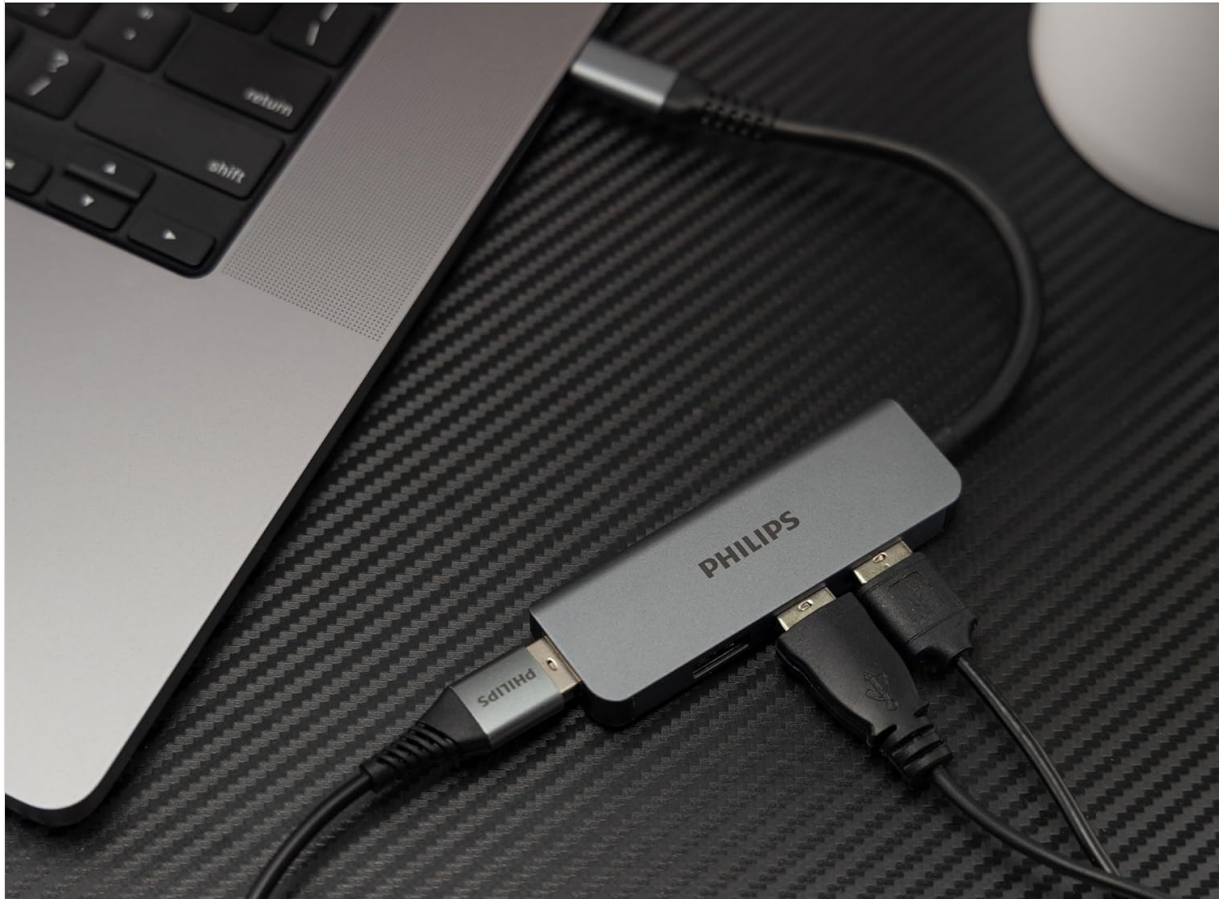
Image 3: Connecting the USB-C Hub to a laptop. This image demonstrates the hub plugged into a laptop's USB-C port, with other USB-A devices connected to the hub.
