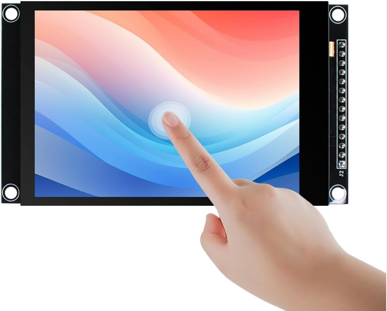
Figure 2: The capacitive touch screen allows direct hand touch, eliminating the need for a stylus.
