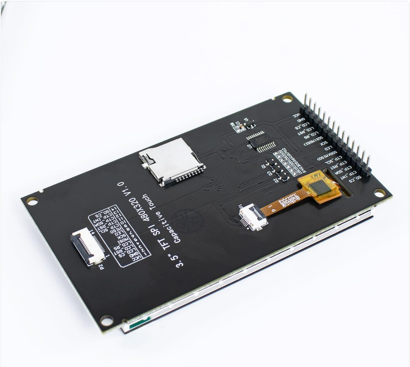
Figure 5: Rear view of the module, highlighting the pin headers and Micro SD card slot.
